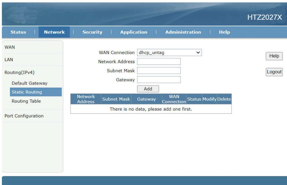
Figure 3-14:Static Routing
