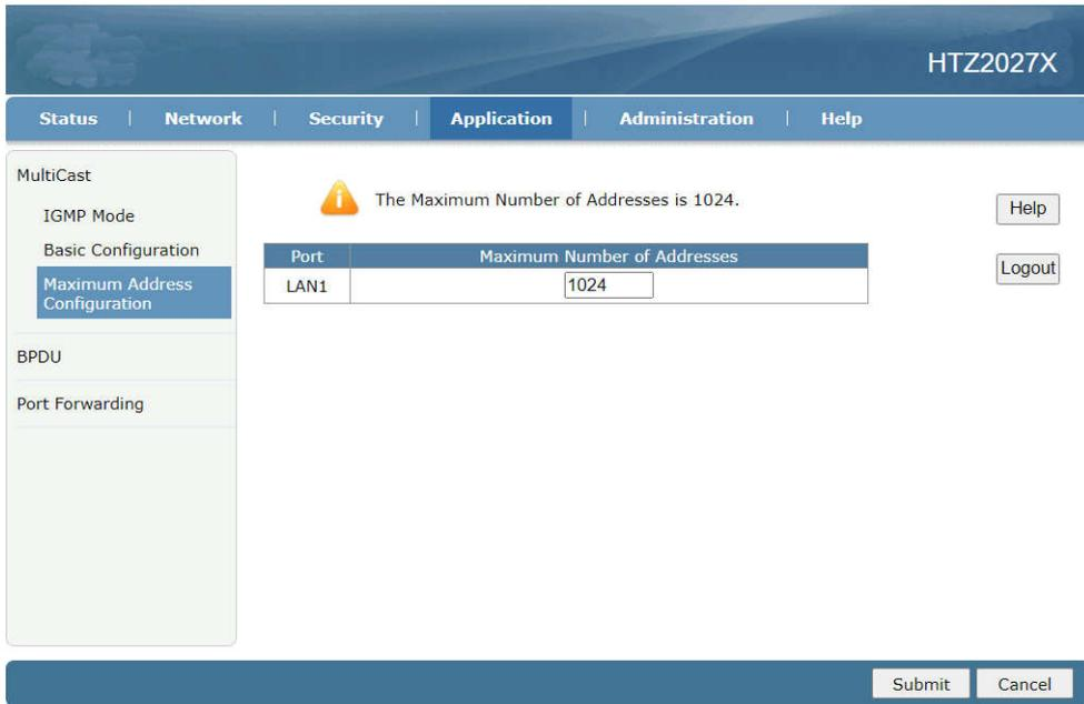
**Figure 3-28: Maximum Address Configuration**
